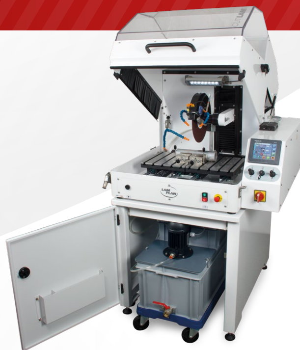
Support cabinet with integrated cooling system (60 litres).
