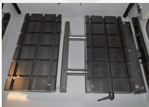
Transversal table X axis 120 mm stroke
